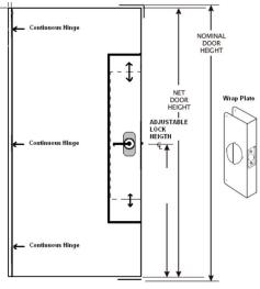
Here's the engineering and a schematic of the components that come into play to make this all possible ...
